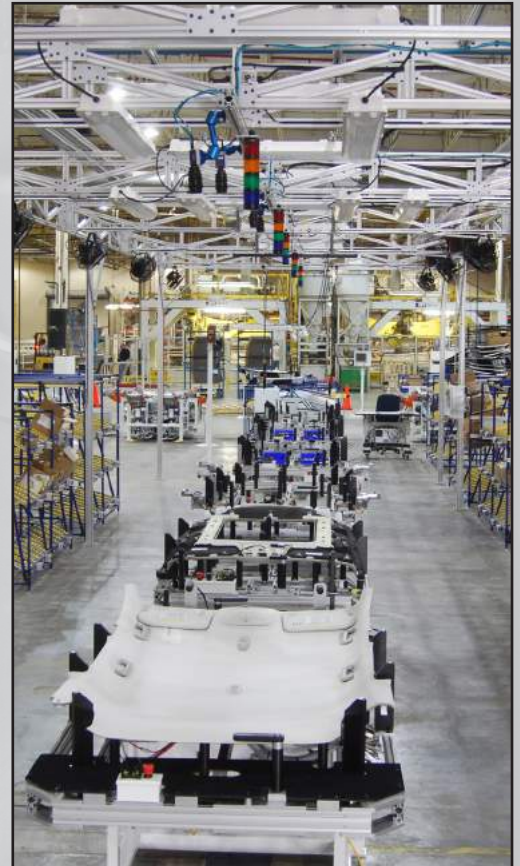
Headliner assembly line with overhead station
